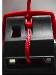
Photo 14. Improperly routed safety cord.
